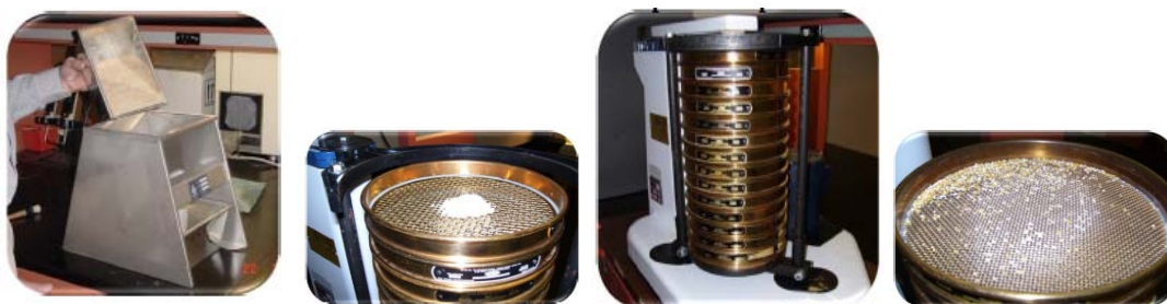
FIGURE 2.4: (a) split sample (b) sample before rotating (c) rotating (d) sample after rotating
