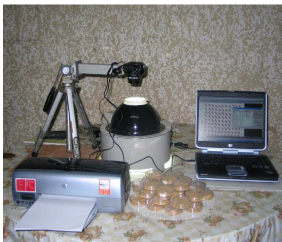
FIGURE 2.6: Pictorial of image acquisition system (Guzman and Peralta 2008)
