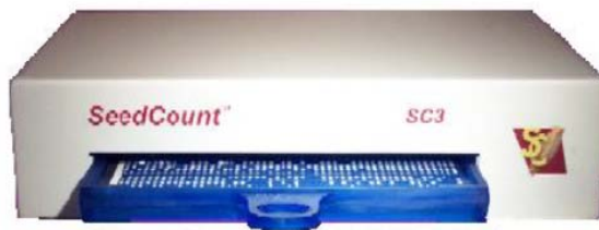
FIGURE 2.5: (b) SeedCount tray in scanner cabinet(Armstrong, et al. 2005)
